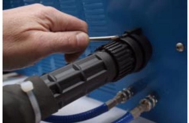
Note that a sealing ring is located in the base of the torch connector socket to form an air seal with the centre power pin. Care should be taken to ensure that this seal is not displaced and that the end of the pin is not damaged when the torch plug is removed.
